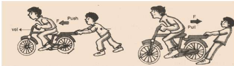
(a) Force exerted in the direction of velocity (b) Force exerted in opposite direction of velocity
